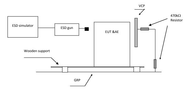
Note: VCP means <u>Vertical Coupling Plane</u> GRP means <u>Ground Reference Plane</u> Wooden support is a 0.1m height rack
