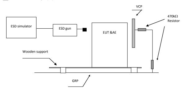
Note: VCP means <u>V</u>ertical <u>C</u>oupling <u>P</u>lane GRP means <u>G</u>round <u>R</u>eference <u>P</u>lane Wooden support is a 0.1m height rack
