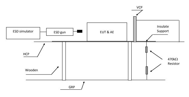
Note: HCP means <u>H</u>orizontal <u>C</u>oupling <u>P</u>lane VCP means <u>V</u>ertical <u>C</u>oupling <u>P</u>lane GRP means <u>G</u>round <u>R</u>eference <u>P</u>lane Wooden support is a 0.8m height table
