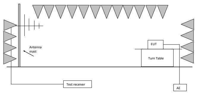
The measurement was applied in a semi-anechoic chamber.
