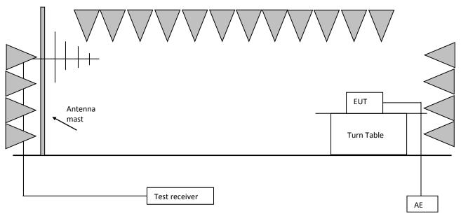
The measurement was applied in a semi-anechoic chamber. Operation conditions of EUT was according to clause 6 of EN 55014-1. Measurement was performed according to clause 10 of CISPR 32. Setting of EUT is according to clause 5.3.4.3 of EN 55014-1. The bandwidth setting on test receiver was 120kHz. The frequency range from 30MHz to 300MHz was checked.
